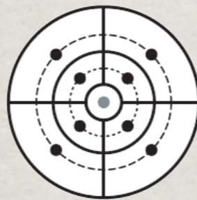
S2: GLOH polar grid with bilinear radial and angular weights
