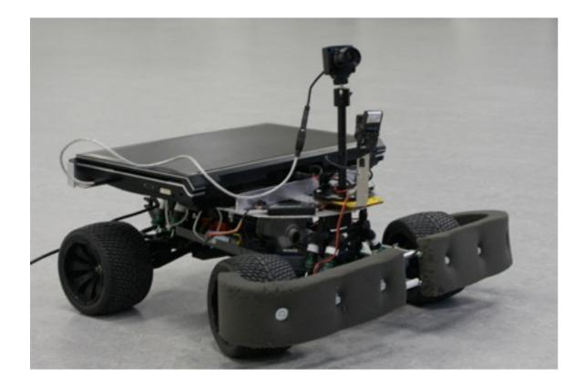
Robot Dog the robot should be able recognize and to follow a specific person.
