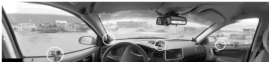
Figure 2.7 Locations of the 4 eye-tracking cameras in the cab of the instrumented vehicle.
