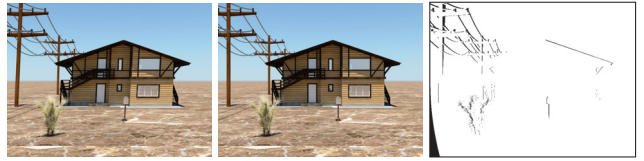
Figure 5. Left to right: Rendered RS frame from sequence of type #2, with N_b = 40 (note that everything is slightly slanted to the right), corresponding global-shutter ground-truth, and mask with white for ground-truth pixels that were seen in the RS frame.
