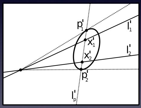
$$\epsilon = 1 - \frac{\max(0, \min(x_h, p_h) - \max(x_l, p_l))}{\max(x_h, p_h) - \min(x_l, p_l)}$$
