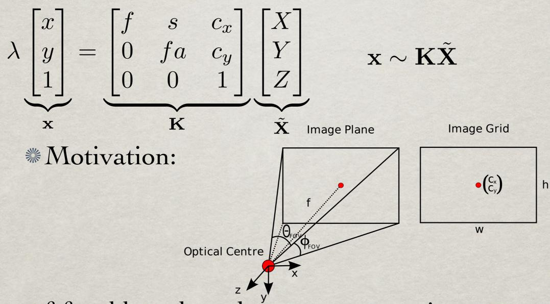
f-focal length, s-skew, a-aspect ratio, c-projection of optical centre
