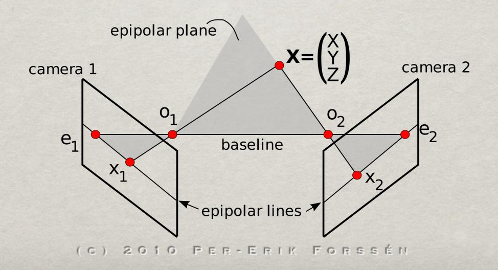
The oriented epipolar constraint compares oriented lines  $\lambda \mathbf{e}_1 \times \mathbf{x}_1$  and  $\mathbf{F}\mathbf{x}_2$
