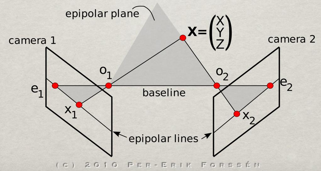
The *oriented epipolar constraint* properly distinguishes points in front and behind of the camera  $\lambda \mathbf{e}_1 \times \mathbf{x}_1 = \mathbf{F}\mathbf{x}_2$ ,  $\lambda \in \mathbb{R}^+$
