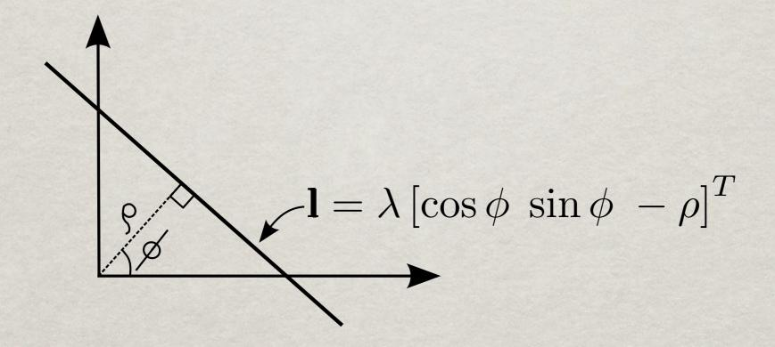
Small amounts of noise in  $x_1$  or  $x_2$  may cause  $\rho$  in  $\lambda e_1 \times x_1$  or  $Fx_2$  to change sign!
