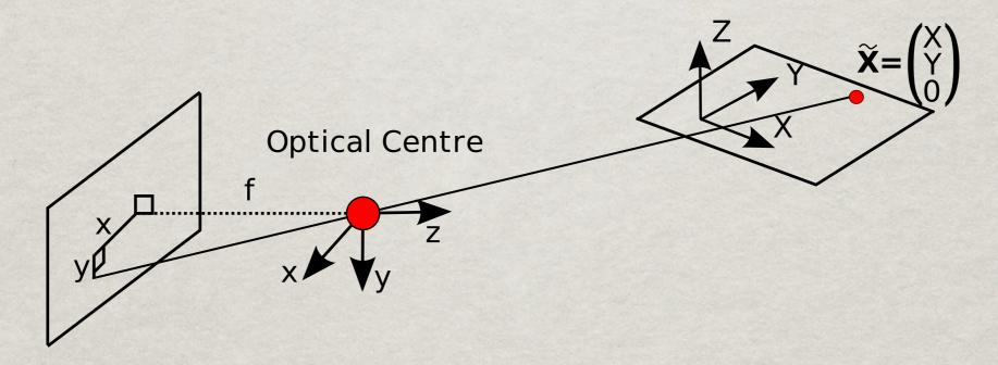
$$\gamma \begin{bmatrix} x \\ y \\ 1 \end{bmatrix} = \mathbf{K} \begin{bmatrix} r_{11} & r_{12} & t_1 \\ r_{21} & r_{22} & t_2 \\ r_{31} & r_{32} & t_3 \end{bmatrix} \begin{bmatrix} X \\ Y \\ 1 \end{bmatrix} = \underbrace{\begin{bmatrix} h_{11} & h_{12} & h_{13} \\ h_{21} & h_{22} & h_{23} \\ h_{31} & h_{32} & h_{33} \end{bmatrix}}_{\mathbf{H}} \begin{bmatrix} X \\ Y \\ 1 \end{bmatrix}$$
