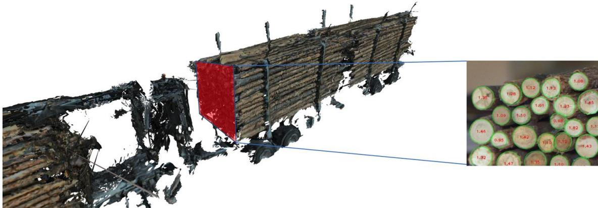
We would like to investigate the possibility to implement our own software for finding and measuring the log ends in order to be independent from the 3<sup>rd</sup> party software. This is a non-trivial task that will require several advanced machine vision technologies and most likely machine learning technologies. The goal is to implement an alternative software and evaluate the performance and accuracy with the existing solution.
