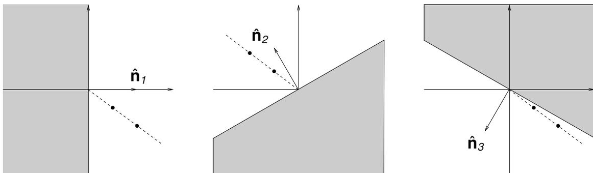
**Figure 17:** Three quadrature filters with directions given by the vectors  $\hat{n}_1, \hat{n}_2, \hat{n}_3$ . The zero half of each filter's Fourier transform is shaded.
