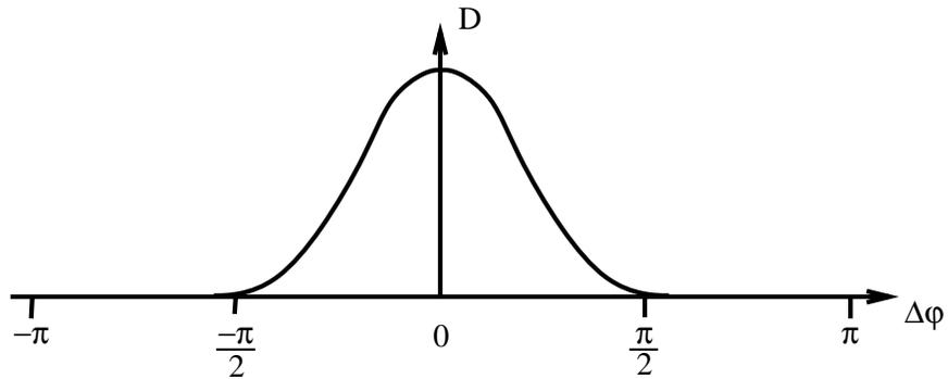
**Figure 3:** One-dimensional plot of the directional function with  $\Delta\phi$ , i.e., the angle between  $\mathbf{u}$  and  $\hat{\mathbf{n}}$ , as parameter.
