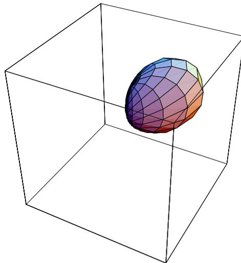
**Figure 4:** Angular plot, i.e., radius =  $D(\hat{\mathbf{u}})$ , of the directional function in 3-dimensional signal space for a particular choice of  $\hat{\mathbf{n}}$ . Origin of the Fourier domain is at the center of the cube.
