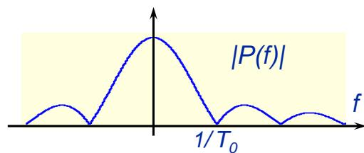
$$p(t) = \text{sinc}\left(\frac{t}{T_0}\right)$$
