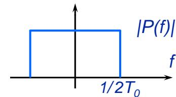
$$p(t) = \frac{\cos(2\beta\pi t/T_0)}{1-(4\beta t/T_0)^2} \text{sinc}\left(\frac{t}{T_0}\right)$$
