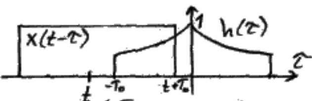
$$y(t) = \int_{-T_0}^{t+T_0} e^{\tau} d\tau = e^{t+T_0} - e^{-T_0}$$
