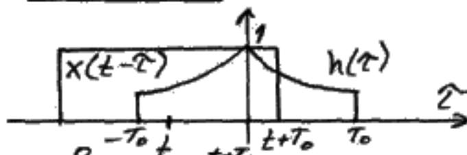
$$y(t) = \int_{-T_0}^{t+T_0} e^{\tau} d\tau + \int_0^{t+T_0} e^{-\tau} d\tau = 2 - e^{-T_0} - e^{-t-T_0}$$
