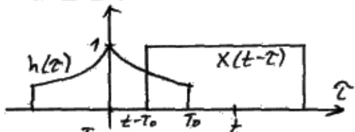
$$y(t) = \int_{t-T_0}^0 e^{\tau} d\tau + \int_0^{T_0} e^{-\tau} d\tau = 2 - e^{t-T_0} - e^{-T_0}$$
