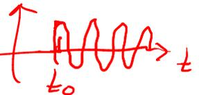
$y_{ps}(t) = \underbrace{y_{transient}(t)}_{h\text{-termen}} + |H(\omega_0)| \cos(\omega_0 t + \arg H(\omega_0)) u(t - t_1)$
