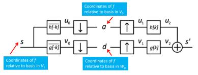
An orthogonal 2-channel filter bank with
