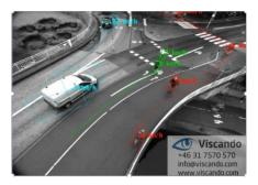
The way we do it is through collecting real time, accurate and objective information about movements, behaviors, interactions, and conflicts of road users using our in-house developed 3D&AI based stationary stereovision sensors. We use this information to yield actionable insights on traffic risks, real-time traffic information, as well as traffic scenarios and behavior models.
