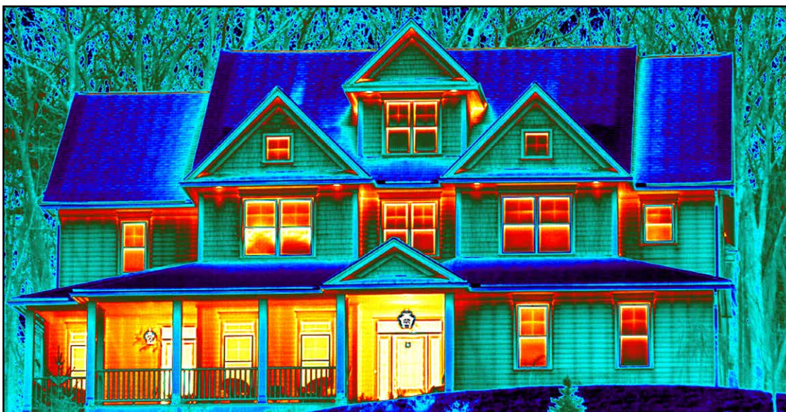
Figure 2: Every thermal image includes materials with different levels of emissivity and reflectivity. Understanding these properties is vital for accurate temperature measurements.
