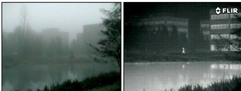
Figure 4: Atmospheric moisture like fog can greatly reduce a thermal camera's detection range. Also note the thermal reflections of the person and building on the surface of the water.
