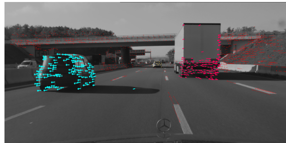
Figure 5: Shire results. Red tracks are world, cyan, yellow and pink are IMOs. The track on the cyan car's shadow causes the IMO bounding box to be significantly extended for the car. This happens because the sun is distant, and the car moves in the plane the shadow is projected on top. A downside of the purely geometric method, as we do not collide with shadows.
