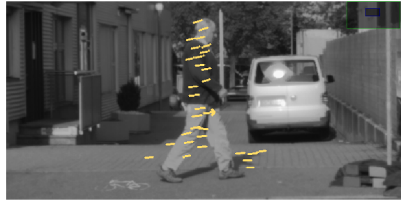
Figure 4: Shire result. A pedestrian IMO detected by the system. While violating the rigid object assumption, people, and most other non rigid IMOs, are often locally rigid. At 100x200 pixels the pedestrian is too small to be fractured into several IMOs. Instead it is intermittently lost and re-detected. The ability to detect generic IMOs is an advantage of the purely geometric method.
