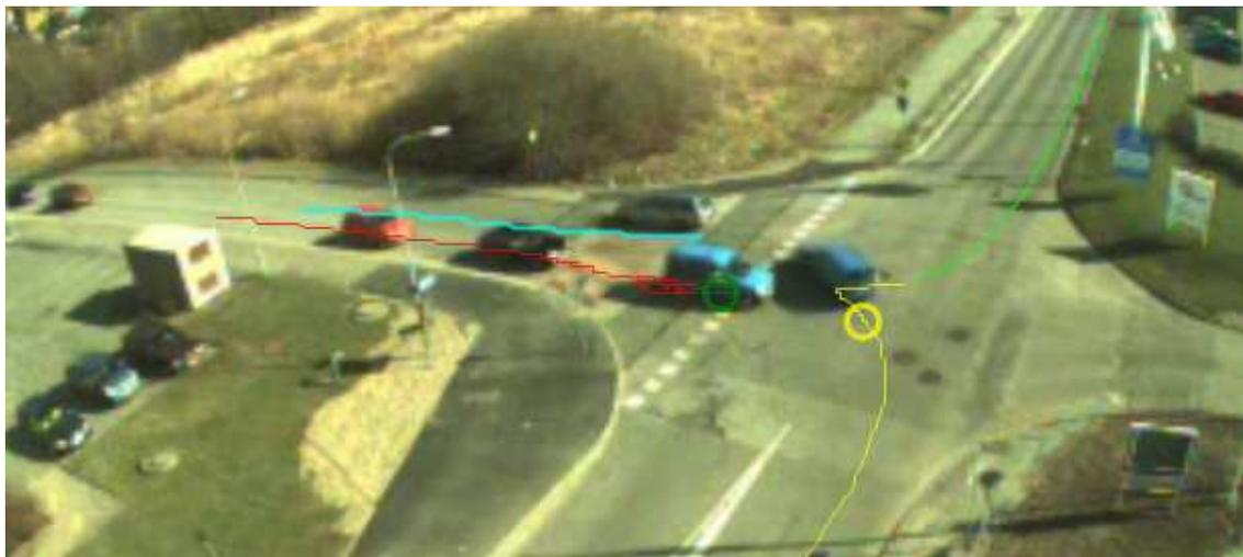
Figure 4a: Trajectories in original data (from coarse image processing), only trajectories representing the two blue vehicles in the centre are shown. The circle indicates the current vehicle position.
