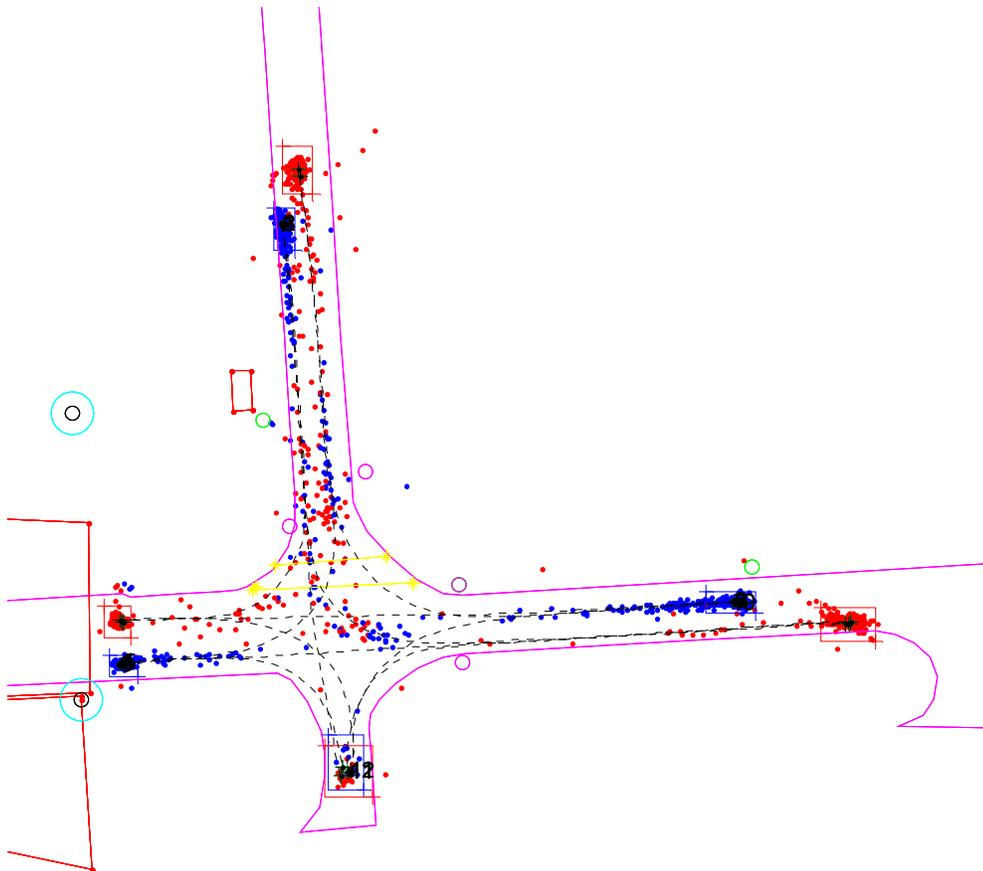
Figure A1: Illustration of using *get\_principals\_advanced.m*. Trajectory entrance points are blue and exit points are red. The boxes are manually entered with two points each. The principal trajectories generated through this process are shown as the dotted black curves. No trajectories were found travelling from south to north, thus no principal trajectory could be generated for this path.
