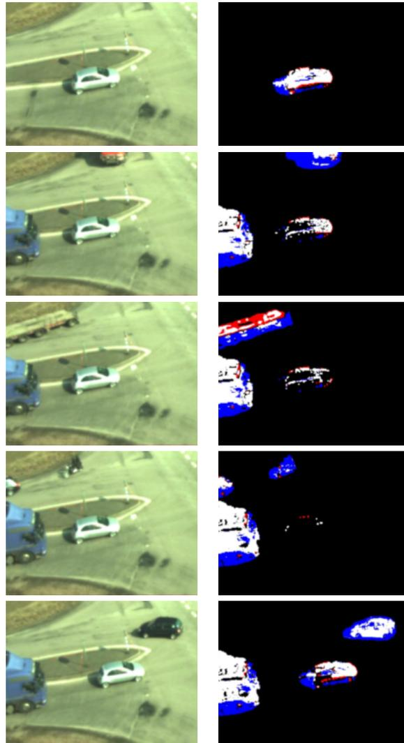
Figure 27: Example of the background model adapting to a vehicle.
