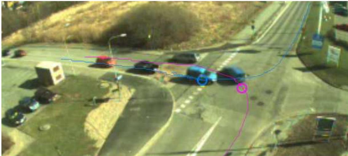
Figure 4c: Trajectories after automatic split and automatic merge (entire automatic repair).
