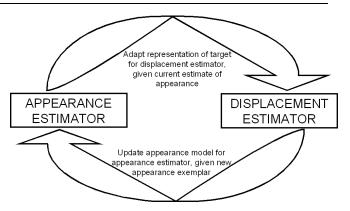
Fig. 1 Simultaneous Modelling and Tracking methodology: The displacement estimator, as well as generating the tracking output, provides a mechanism for supervision of the appearance model learning process *i.e.* it provides new examples of the target appearance that are added to the appearance model. In return, the appearance estimator provides information about the structure of the target appearance space that enables the tracker to cope with a high degree of variation in appearance.
