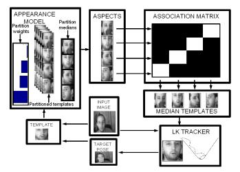
Fig. 8 *LK-SMAT system architecture*: The SMAT appearance model identifies aspects by partitioning templates using a greedy clustering algorithm. Identifying the current aspect selects the template for use in registration process. The association matrix in this formulation is simply an identity matrix.
