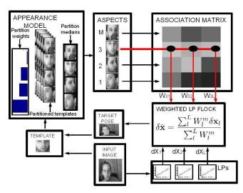
**Fig. 9** *LP-SMAT system architecture*: LPs associated to the active SMAT appearance model component through association matrix are activated for tracking. The contribution each LP makes is determined by its strength of association with the current aspect. Association strengths are updated to reflect the LP's performance for the current aspect each frame.
