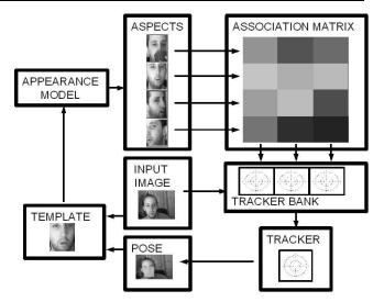
Fig. 2 Generic system architecture: The appearance model stores all target templates and identifies aspects of the target. Aspects are associated to feature trackers by an association matrix. Each feature tracker contributes to the overall pose estimation, the level of contribution is determined by the strength of association to the current aspect *i.e.* the association matrix value.
