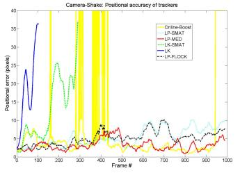
Fig. 23 The positional error for each tracker is shown. Where the Online-Boost tracker fails and is re-initialised is indicated by the vertical yellow lines.
