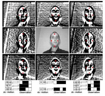
Fig. 5 Intensity difference images for eight translations. Four support pixel locations illustrate the predictive potential of the difference image. The input image is in the center. All images to the left/right of the input have been translated left/right by 10 pixels. Those images above/below the input have been translated by 10 pixels up/down. Under the images, the motion and support vectors are illustrated.
