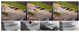
**Fig. 15** Tracking results for LP-MED (solid rectangle) and Online-Boost (dashed rectangle) are shown for first, last and middle frame of sequence along with the median templates identified by the SMAT appearance model during frame 141.
