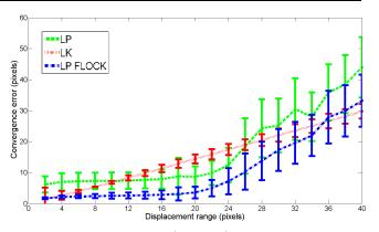
Fig. 11 Convergence error (in pixels) for three tracking approaches over a range of test displacements. The error bars represent the log of the variance of the pixel error over the 3000 tests at each range.
