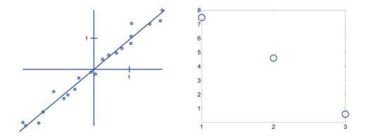
Figure 11.7: Left: the same point set as in Figure 11.3 after a H-normalization. This figure also shows the line that is estimated by algebraic minimization based on the homogeneous method. Right: the singular values of the corresponding data matrix.
